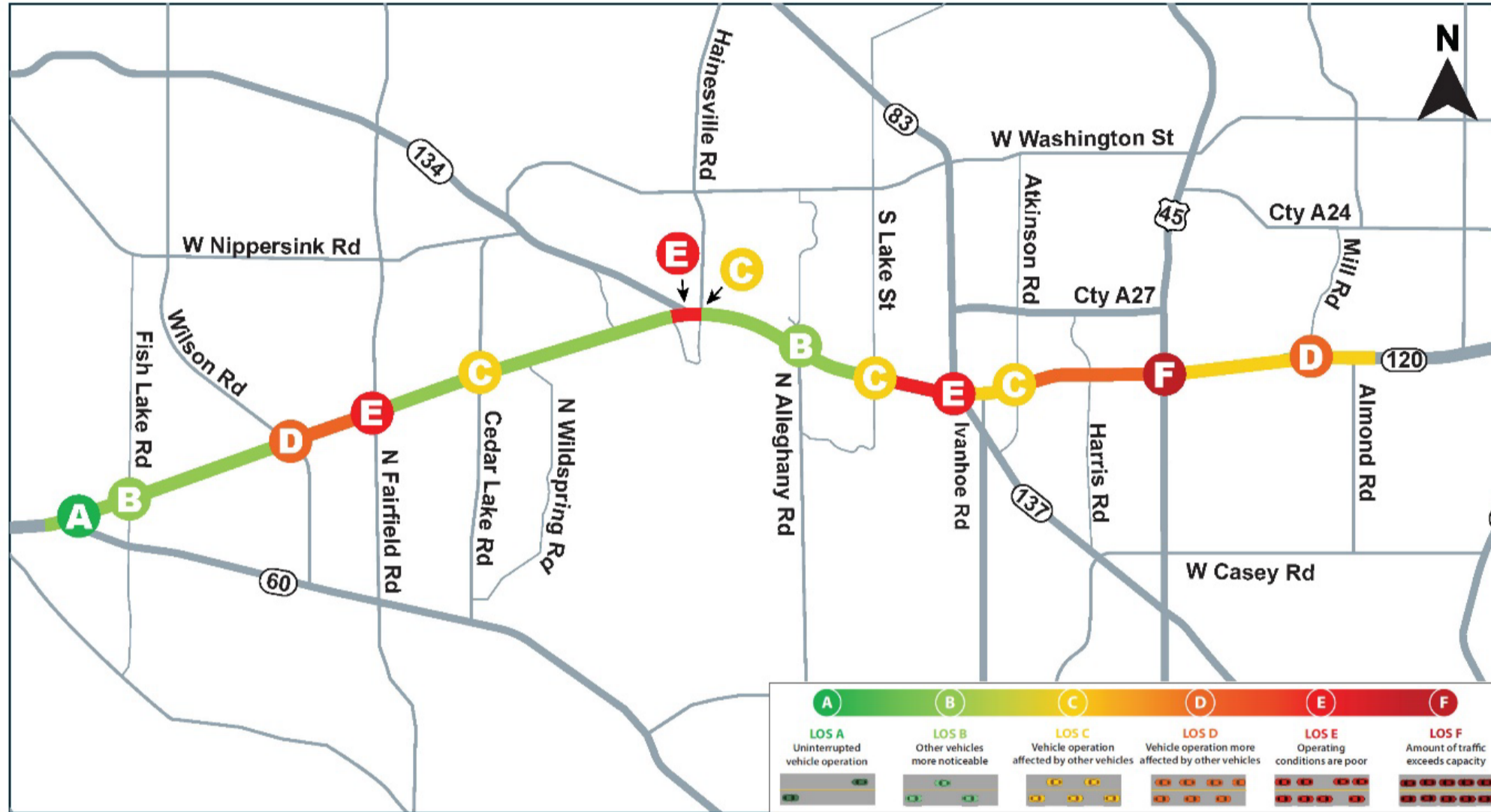
NO BUILD 2050 LEVEL OF SERVICE (A.M.) IL 120 FROM IL ROUTE 60 TO ALMOND ROAD
