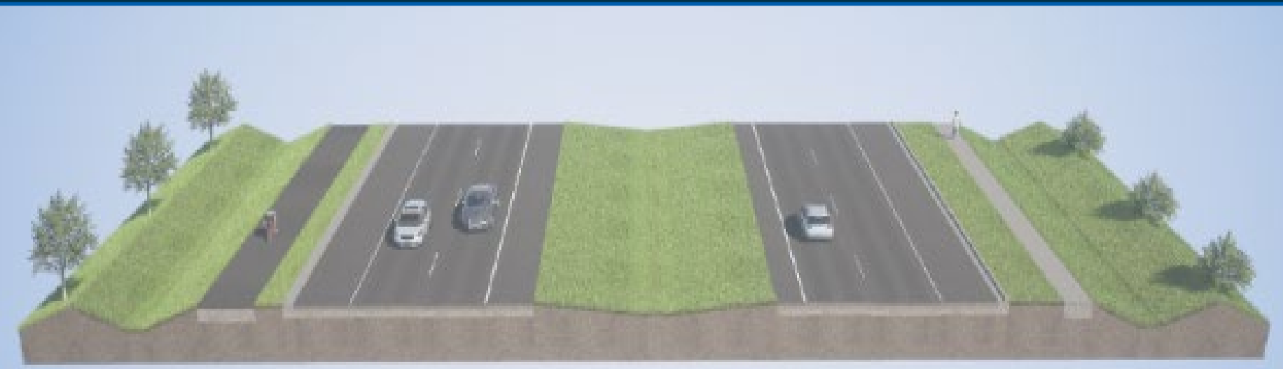
Principal Arterial – 5 Lane Rural
